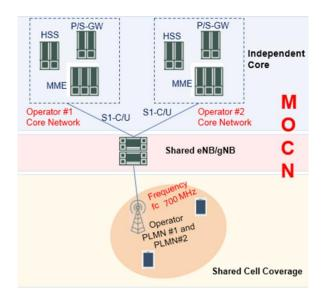
Figure 2.3: Multi-Operator Core Networks
