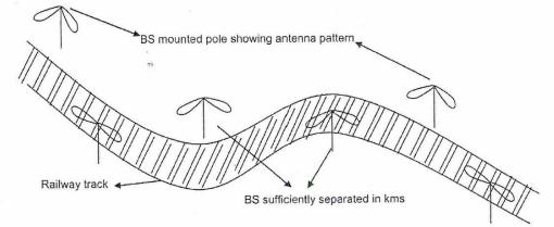
Fig. 12 - LTE eNBs along the Railway Track with Antenna Boresight Focusing the Track
